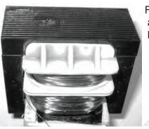
For small commercial transformers, the coils are placed around the centre pillar of the core, which is shaped like this:
