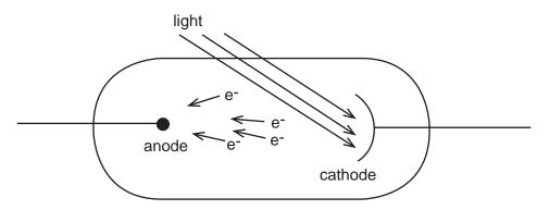
The photocell works when incident light falls on a metal cathode and causes electrons to be ejected with a certain kinetic energy from the metal. These electrons then move across the cell to the anode. The kinetic energy of an ejected electron is equal to the energy of the incident light minus the work function W (the energy required to remove the electron from the metal).
