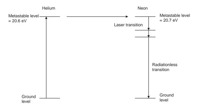
A mixture of helium and neon gas at low pressure is placed into a glass tube. An electric discharge in the gas excites the helium atoms, which then collide with the neon atoms, exciting them. Photons produced in spontaneous emission initiate stimulated emission and amplification of the laser transition begins.
